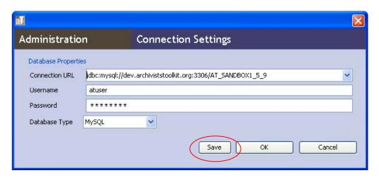
Enter the database properties and click on the 'save' button. When the connection settings window is opened again, the drop-down menu will display all Connection URLs that have been previously saved.
